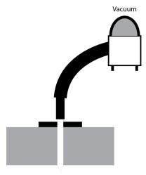
Do **not** ream the hole. Do **not** make the hole any wider than the drill bit made it.
