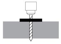
Use a carbide bit (conforming to ANSI B212.15-1994).
