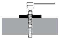
**Important**: Do *not* use an impact wrench to torque the Anchor Bolts.
