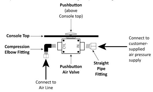
Drawing not necessarily to scale. Not all components shown. Pushbutton is above the Console top, all other components are under the Console top.
