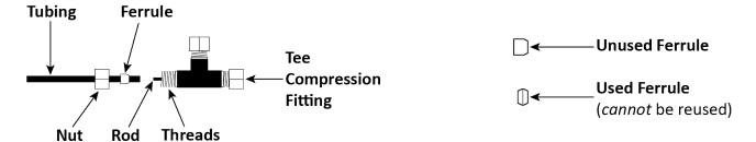
**Important**: *Ferrules can only be tightened once*. When you tighten the Nut on the Threads, the Ferrule gets compressed; it literally changes shape and *cannot* be used again.
