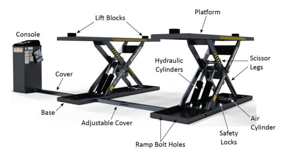
MDS-6EXT shown without Ramps. Power Unit and Flow Divider are inside the Console. Air and Hydraulic Lines are routed under the two Covers.
