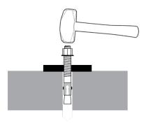
Even using a hammer or mallet, the Anchor Bolt should only go into the hole part of the way; this is normal. If the Anchor Bolt goes all the way in with little or no resistance, the hole is too wide.
