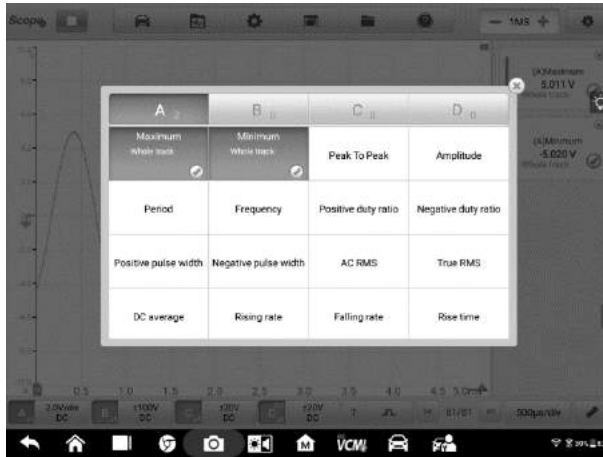
Figure 7-82 Sample Measurement Setting Screen
