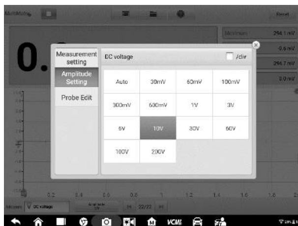
Figure 7-17 Amplitude Setting Screen (DC 10V)
