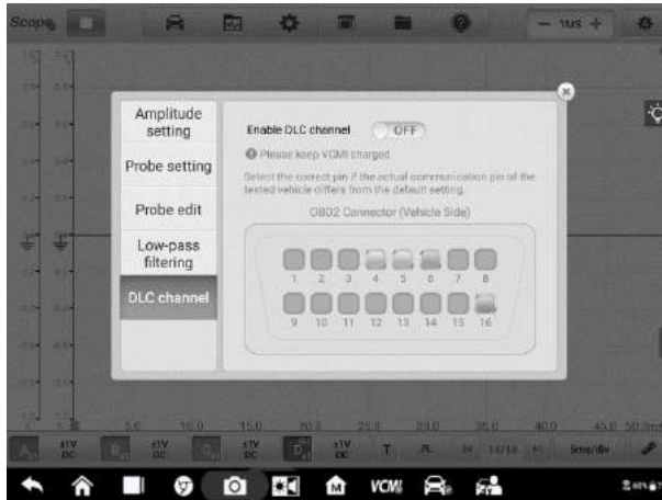
Figure 7-61 Sample DLC Channel Setting Screen 1
