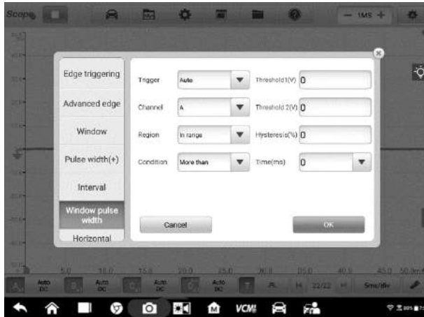
Figure 7-73 Sample Window Pulse Width Settings Screen
