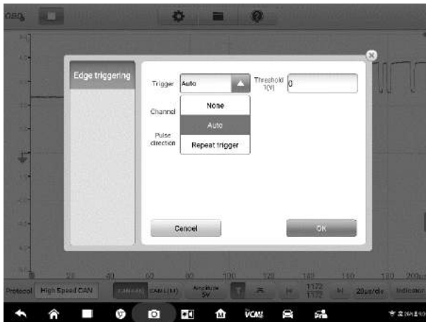
Figure 7-23 Sample Trigger Mode Screen
