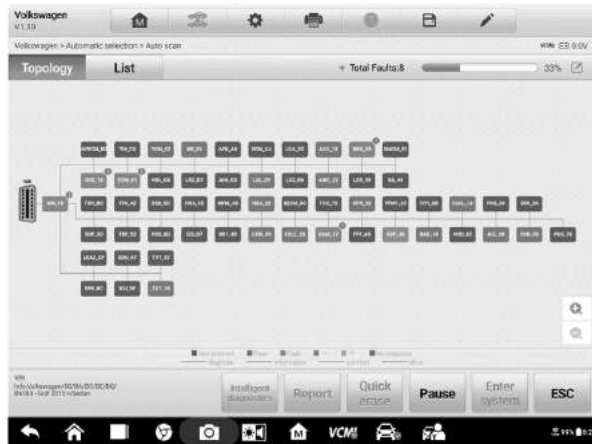
Figure 5-6 Sample Fault Scan on Topology Screen
