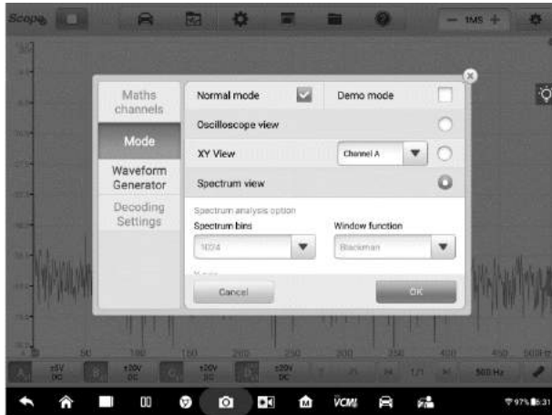
Figure 7-84 Sample Spectrum View Selection Screen
