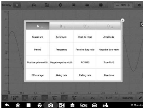
Figure 7-80 Sample Measurement Screen 1
