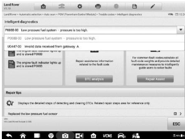
Figure 5-16 Sample Vehicle System and Detected DTC(s) Screen
