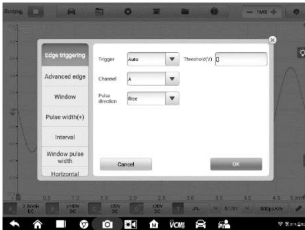
Figure 7-65 Sample Trigger Settings Screen
