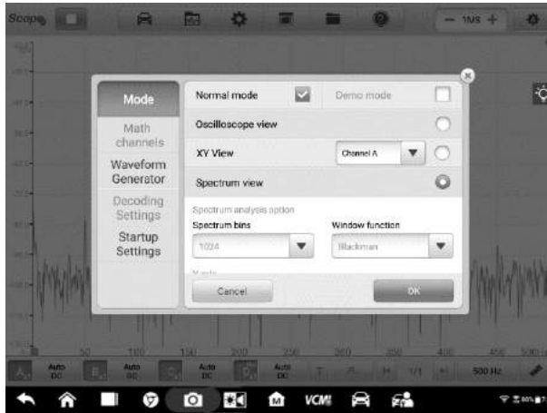
Figure 7-17 Sample Spectrum View Setting Screen 1
