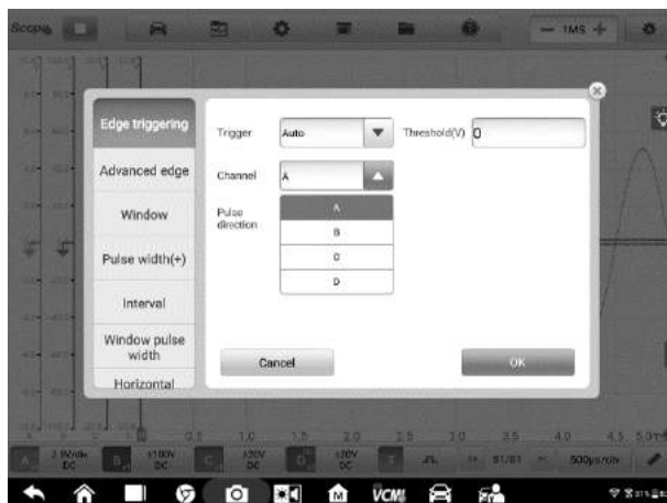
Figure 7-67 Sample Trigger Channel Screen
