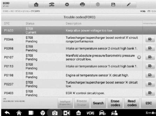
Figure 4-29 Sample DTC & FFD Screen
