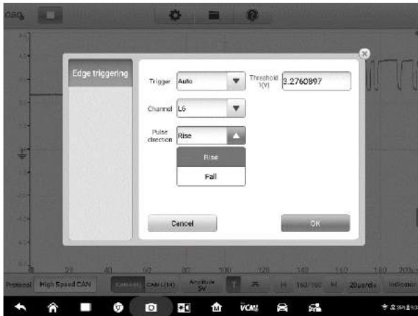
Figure 7-24 Sample Pulse Direction Screen
