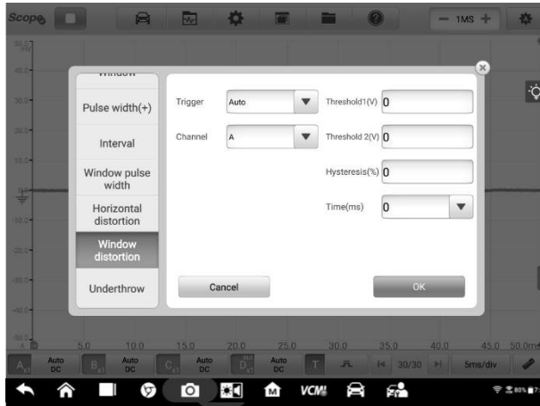
Figure 7-75 Sample Window Distortion Settings Screen
