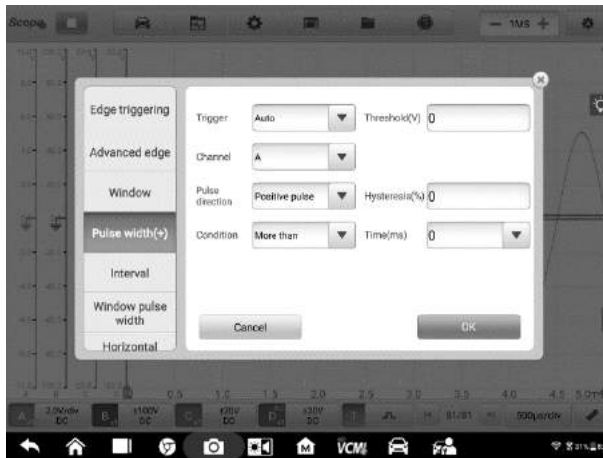
Figure 7-71 Sample Pulse Width Settings Screen
