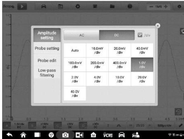
Figure 7-51 Sample Amplitude Setting Screen (DC 1.0V/div)
