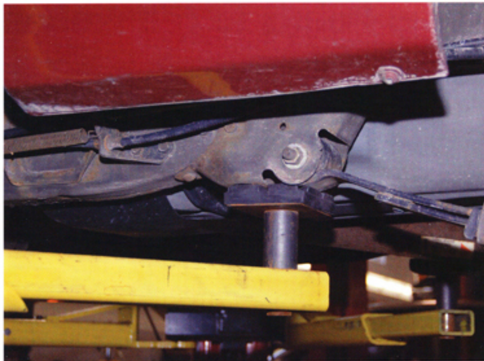
Adapter in contact with hanger only. OK TO LIFT HERE.
